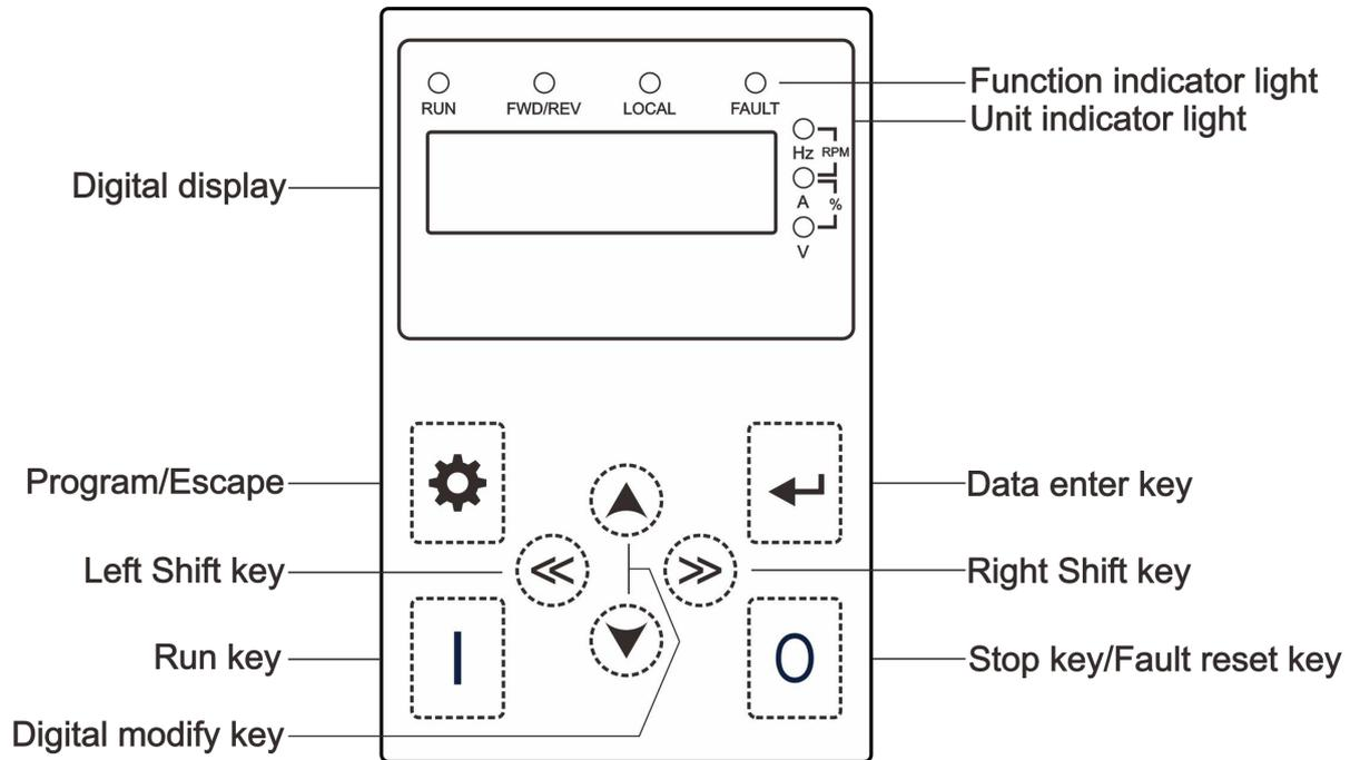
Figure 5.1.1 Keypad schematic diagram
