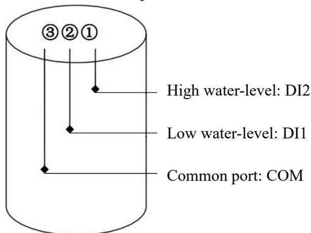
Figure 4.4.5 The wiring for water-level sensors in the well
