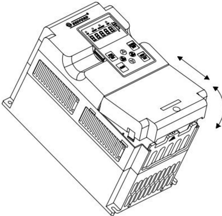
Figure 3.2.1 Disassembly and installation of plastic
