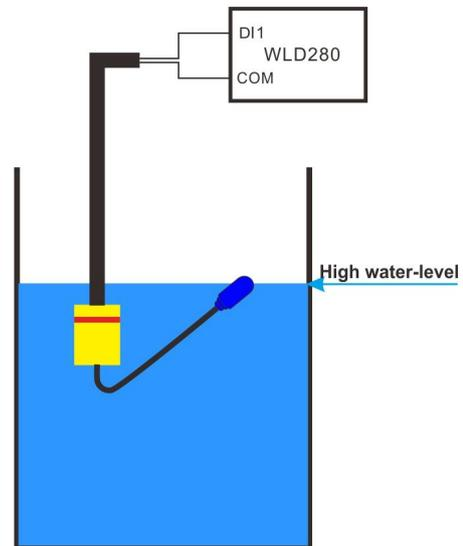
Figure 4.4.2 The high water-level
