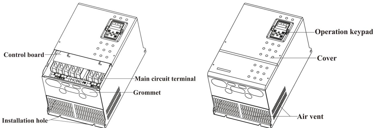
Figure 2.5.2 Parts of controllers (220V: 30kW and above, 380V: 45kW and above)
