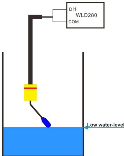
Figure 4.4.1 The low water-level
