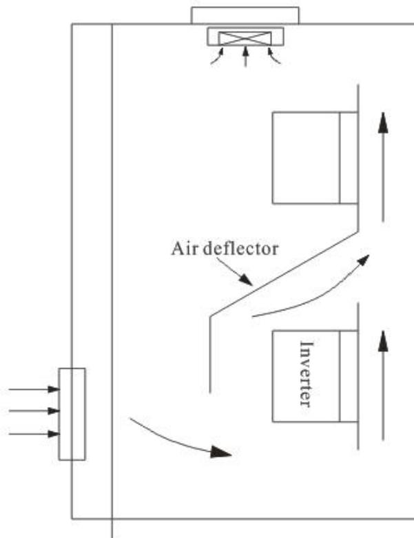
Figure 3.1.2 Installation of multiple controllers
