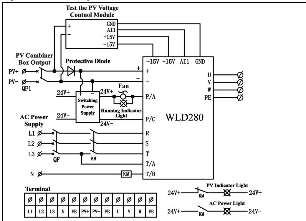
Figure 4.3.1 Inverter AC/DC switching
