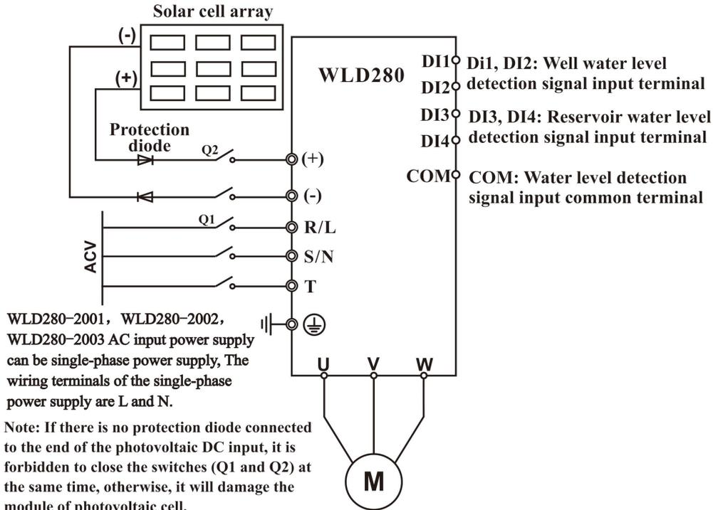
Figure 4.2.1 The solar cell array and the power frequency power supply wiring diagram
