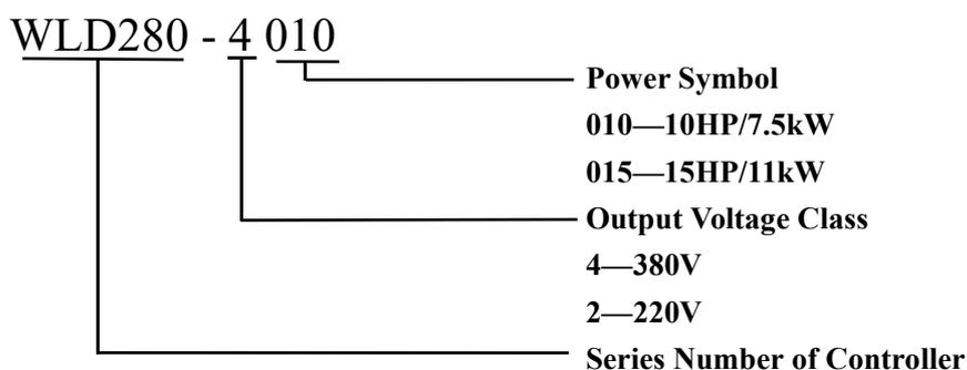
Figure 2.3.1 Nameplate of controller
