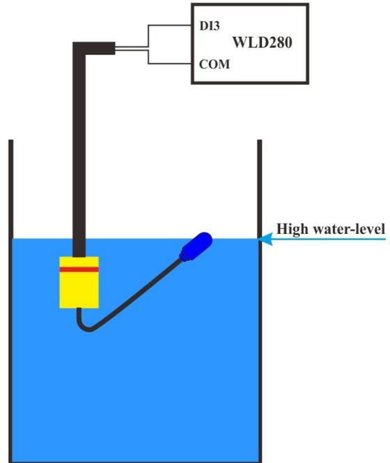
Figure 4.4.7 High water-level
