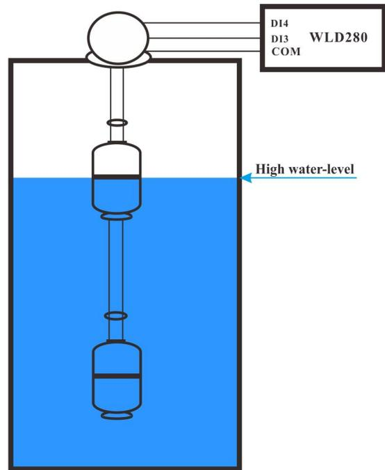
Figure 4.4.9 High water-level
