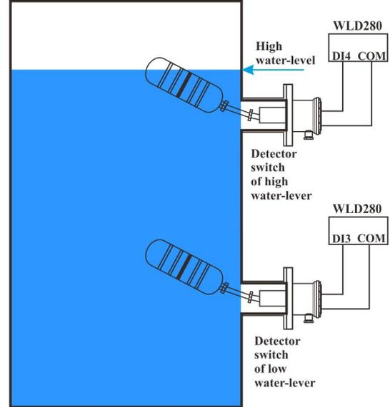
Figure 4.4.12 High water-level
