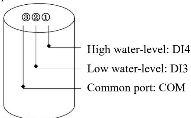
Figure 4.4.10 The wiring for water-level sensors in the well
