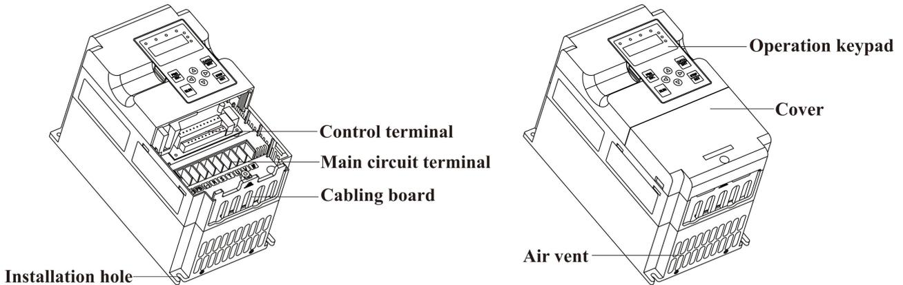
Figure 2.5.1 Parts of controllers (220V: 22.0kW and below, 380V: 37.0kW and below)
