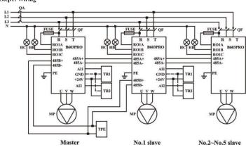
Control 5 auxiliaries at most, up to 6 pump linkage work
